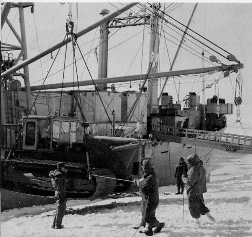
HEAVY-DUTY tractor is lowered over side of the WYANDOT onto the ice shelf to act as conveyance, trailer haul, and bulldozer. Moderate uphill grade posed few problems but hazards were there.
