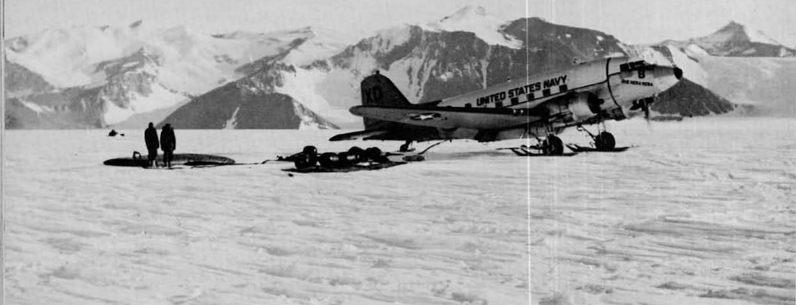
PUMPING FUEL FROM R4D INTO STORAGE TANK NEAR BEARDMORE GLACIER FOR REFUELING RETURN POLAR PLANES.
