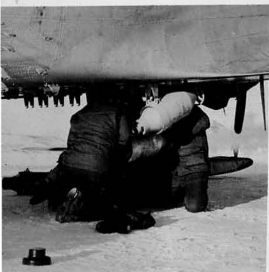
MOUNTING JATO BOTTLES ON R4D (LEFT); MOTOR REPAIRS INSIDE HEATED OUTDOOR "HANGAR" ON SKYMASTER.
