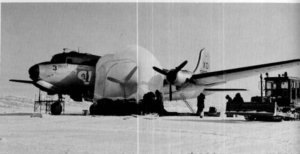
MOUNTING JATO BOTTLES ON R4D (LEFT); MOTOR REPAIRS INSIDE HEATED OUTDOOR "HANGAR" ON SKYMASTER.
