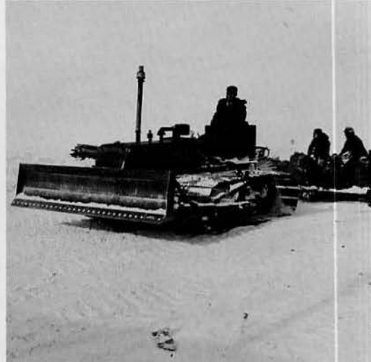
HARVESTING SNOW FOR THE MELTER HAS BEEN REDUCED TO A SCIENCE THANKS TO PARACHUTE BAGS AND TRACTORS.
