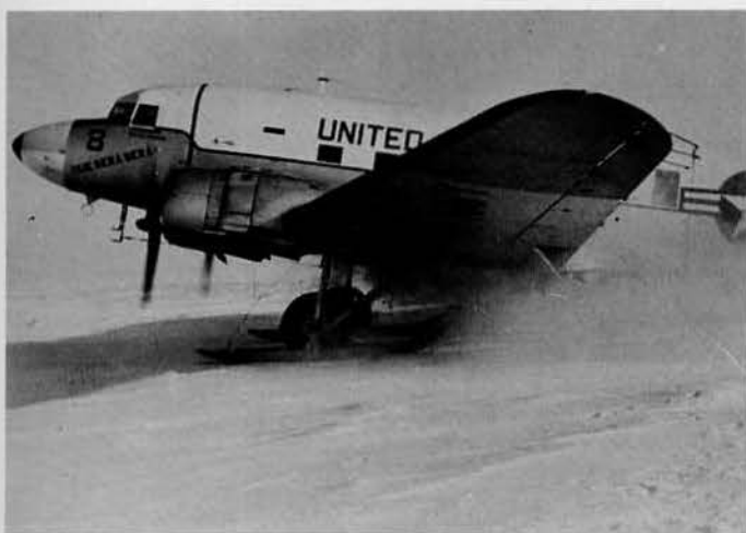
ON DECK at the pole, the historic plane keeps its motors cranking to avoid hazardous freeze-up in minus 58° cold.
