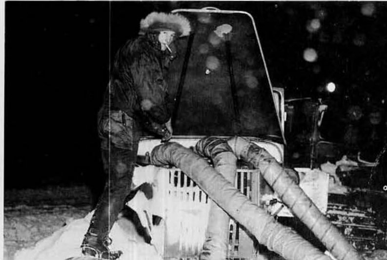
"warehouses." Balky SnoCat gets preheating treatment for one last sortie into a twilight snowstorm at LA-V.
